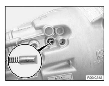
Force open bearing bushing (1) and withdraw using a suitable tool.
