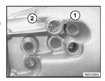
Remove pressure spring and locking pin.
