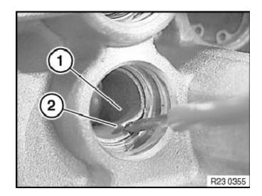
Drive in bearing bushing (1) with special tool (see table).
